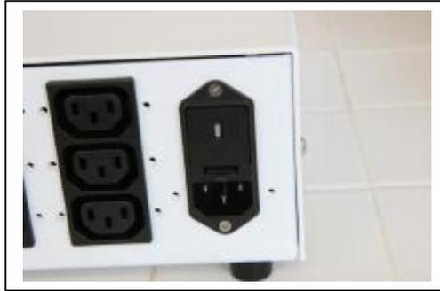
Use a small screw driver, or such, to lift and release the tab securing the fuse holder in place.
