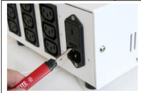
Remove the fuse holder and put it aside.
