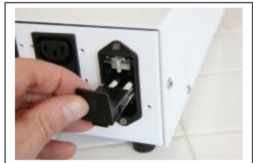
Locate the voltage selector card inside power entry module on the IsoBox (gray piece with a 3 digit number representing the selected voltage). Remove the Voltage Selector card using the same screw driver by prying/pulling it straight out.
