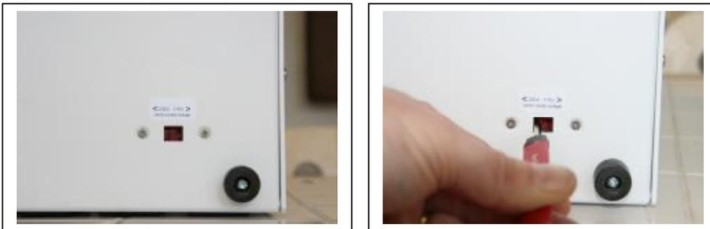
For an additional verification, we recommend hooking up the transformer to intended input power without any equipment connected to output, and verify output voltage using a voltage meter. Incorrect voltage settings can cause extensive damage and possible harm to persons.
