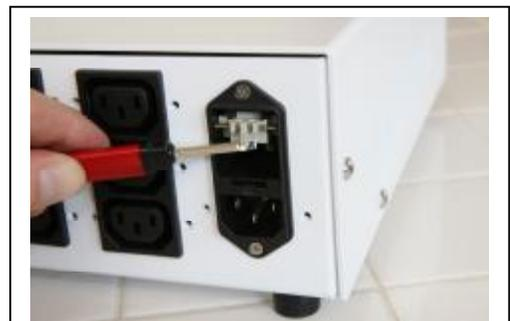
Look at the voltage selector card and chose the input voltage you need (number represent voltage selection). This number should be visible outward when the card is inserted again into the power entry module. Insert card and push it in hard until it stops.
