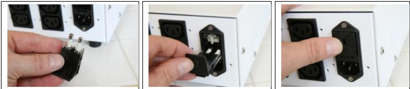
The output voltage can be verified and changed also. Turn the IsoBox onto its side. Locate the rectangular hole. The label should indicate the direction which the switch should slide for the correct voltage. You can change by using a small screw driver, like the one used for the input voltage. VERIFY by looking into the hole and be assured the correct voltage is visible.
